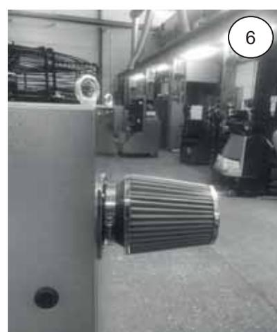
Once the collar is tight, the air filter is properly installed.
