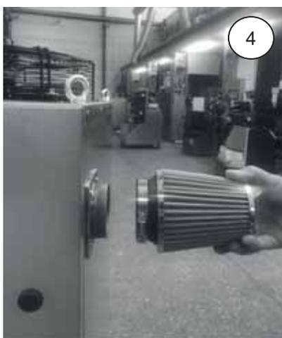
Place the filter on the air duct.
