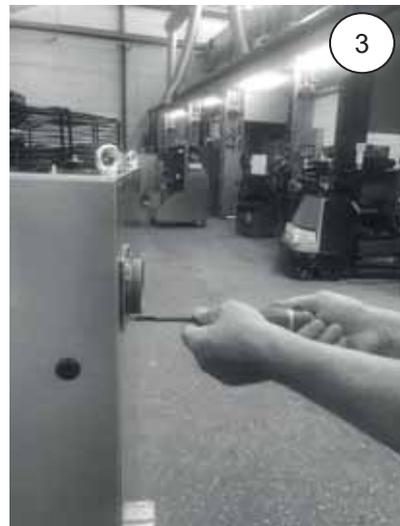
Secure the duct with the 4 screws provided and a screwdriver.
