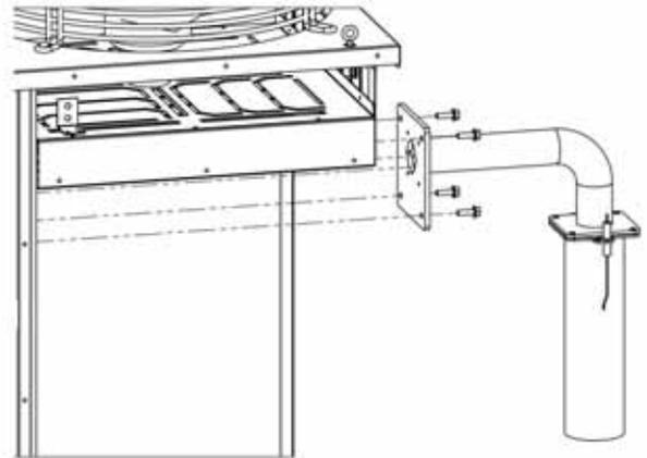
5°/ Remove the burner assembly, fig.3 / 4:
