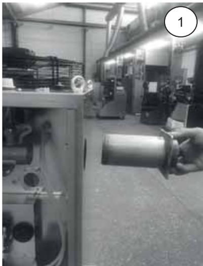
Insert the air duct into the hole provided for this purpose on the upper side of the appliance.
